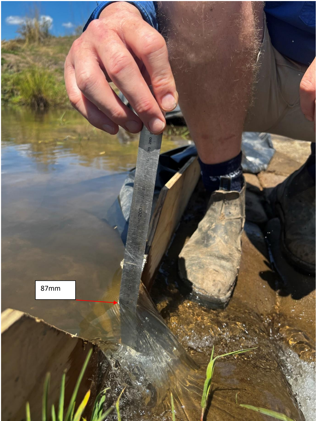
Figure 10 V-notch weir measurement
